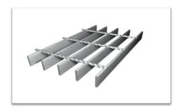
Safegrid / Flowforge "W" steel grating comprises of a series of parallel, flat, load bearing bars at equal spacing. These are held upright by 6mm twistedsquare transverse bars that are resistance welded into the top surface.
