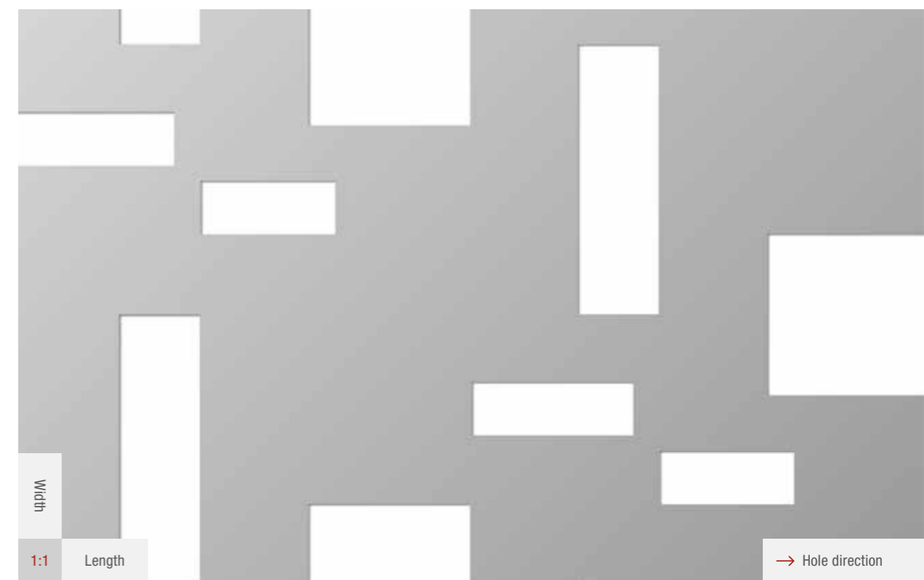
RMIG INFINITY Hole from 10 to 50 Open area 25.9 %
